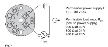
Note that twisted leads must be used for the output signal.
